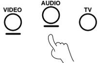
Press the **VIDEO**, **AUDIO**, or **TV** key to select the input you want to register. (Each press of the key advances you one by one through the available input settings.) The current input setting appears on the display of the receiver.
