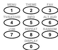
Use the numeric keys to enter the 4-digit setup code for the component.
